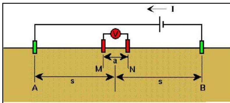
Figure 3: Schlumberger Array for Data Acquisition
